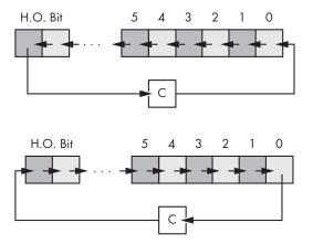
Figure 2-17: rcl(1, dest) and rcr(1, dest) operations
