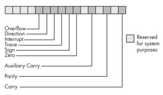
Figure 2-20: EFLAGS register as packed boolean data
