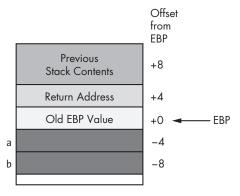
Figure 5-6: Activation record for the LocalVars procedure
