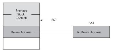
Figure 5-2: Stack contents before ret in messedUpToo
