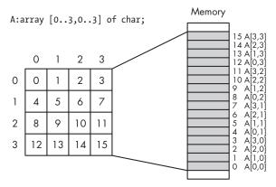
Figure 4-9: Column-major array element ordering
