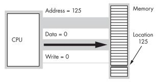
Figure 1-7: Memory write operation
