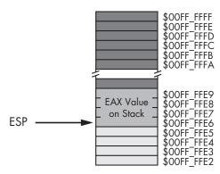
Figure 3-13: Stack after pushing EAX
