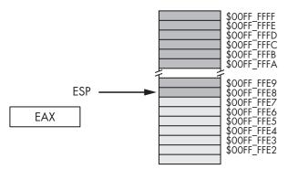
Figure 3-9: Stack segment before the push( eax ); operation
