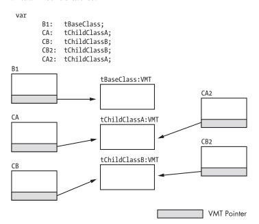
Figure 12-7: Virtual method table references from objects
