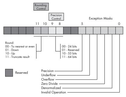
Figure 6-2: FPU control register
