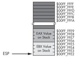
Figure 3-14: Stack after pushing EBX
