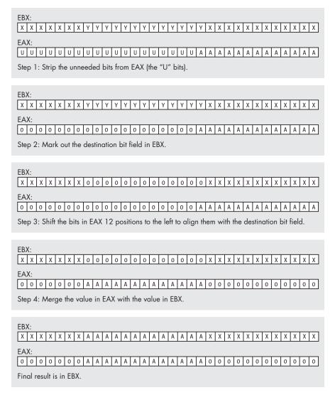
Figure 10-2: Inserting bits 0..12 of EAX into bits 12..24 of EBX
