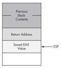
Figure 5-1: Stack contents before ret in MessedUp procedure
