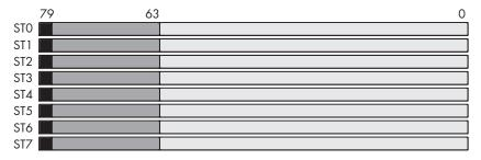
Figure 6-1: FPU floating-point register stack
