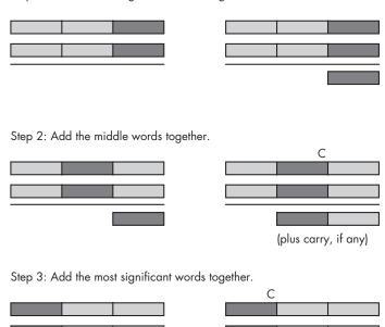
Figure 8-1: Adding two 96-bit objects together
