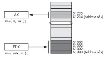
Figure 3-2: Accessing a word or dword using the displacement-only addressing mode
