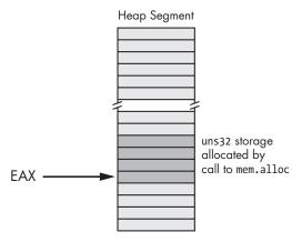
Figure 3-20: A call to mem.alloc returns a pointer in the EAX register.
