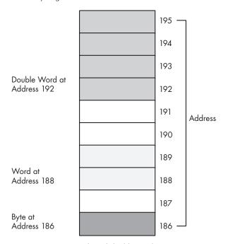
Figure 1-9: Byte, word, and double-word storage in memory
