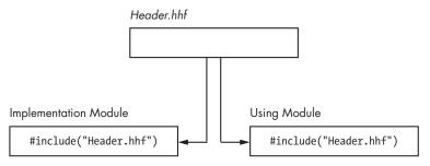
Figure 5-10: Using header files in HLA programs
