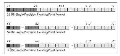
Figure 6-4: FPU floating-point formats
