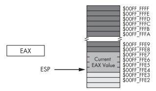
Figure 3-10: Stack segment after the push( eax ); operation
