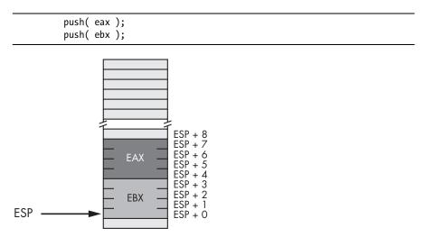
Figure 3-19: Stack after pushing EAX and EBX
