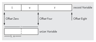
Figure 4-11: Layout of a union versus a record variable
