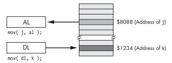
Figure 3-1: Displacement-only (direct) addressing mode
