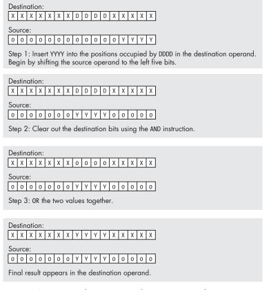
Figure 10-3: Inserting a bit string into a destination operand
