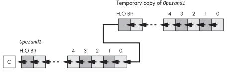
Figure 8-6: shld operation
