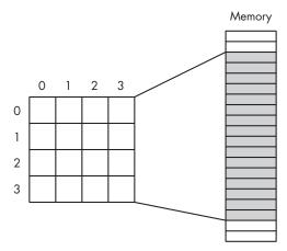
Figure 4-5: Mapping a 4×4 array to sequential memory locations
