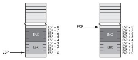
Figure 3-17: Removing data from the stack, before add(8, esp);
