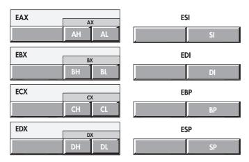
Figure 1-5: 80x86 (Intel CPU) general-purpose registers
