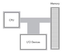
Figure 1-4: Von Neumann computer system block diagram
