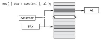
Figure 3-4: Indexed addressing mode using a register plus a constant
